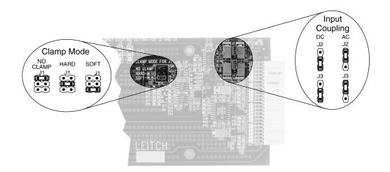
Figure 8-11. VPD-6830-DEQ Jumper Locations
